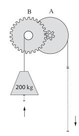
Let's feel our way with conversion factors. We know that one tooth of gear B moves forward after contacting one tooth of gear A, so we can use this to determine the ratio of revolutions of gear B to gear A.
